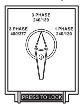
Figure 15. Voltage Selector Switch
